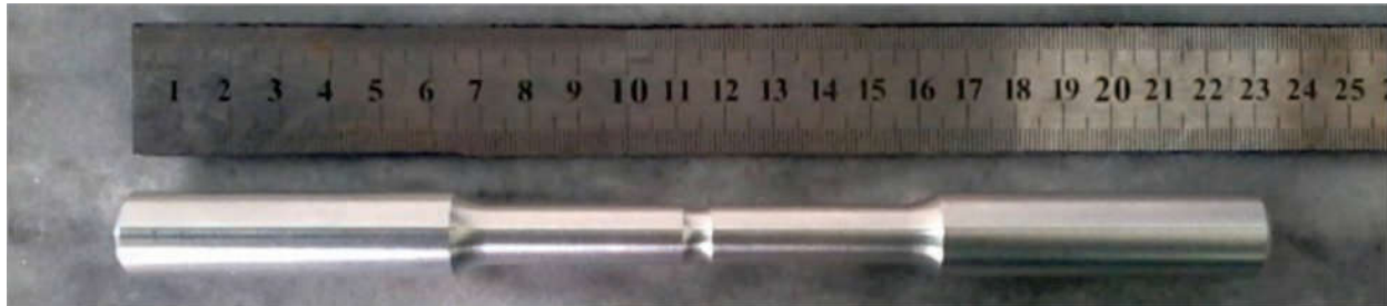
Fig. 1. Picture of the specimen prepared by turning operation.
